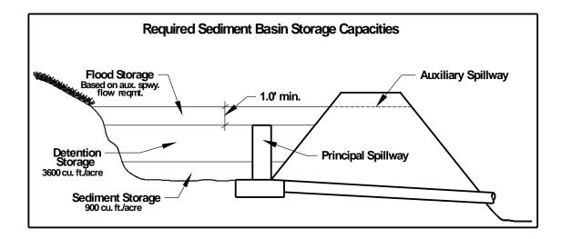
Flood storage is based on the required design storm for the auxiliary spillways. Flood storage is calculated between the crest of the principal spillway and the crest of the auxiliary spillway. A minimum of 1 foot in elevation is required between the principal and auxiliary spillways.
