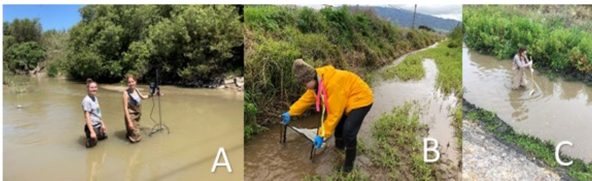
Figure 18. A) Riley Ransom and Yulia Loshkareva preparing to sample microplastic on the Salinas River, with the net submerged to the top of the net opening. B) Riley Ransom collecting a sample at Quail Creek, holding the net in place so that it barely touches the bottom of the creek. C) Jordin Simmons walking upstream holding a net in front of her, collecting a sample at Merritt Ditch, during no-flow conditions.
